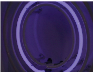
Cold Cathode tubes being driven by LM400D dimming programmable controller.
